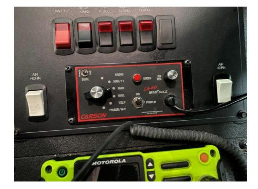
1.7) Dual rocker-style air horn switches mounted in cab console to match below
